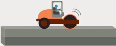
The ash is laid down, layer by layer, and compacted by roller compactors that use both weight and vibration to create a pavement-like hardness.
