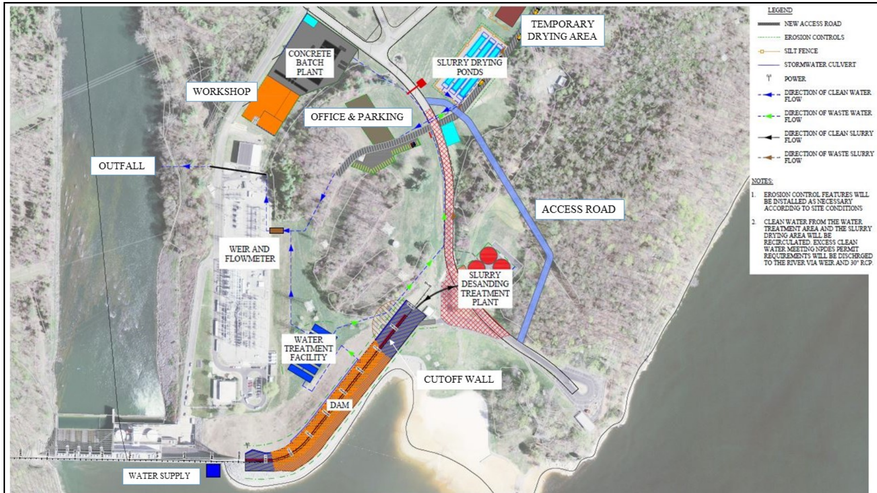
Figure 2-4. Construction Site Plan and Water Flows.
