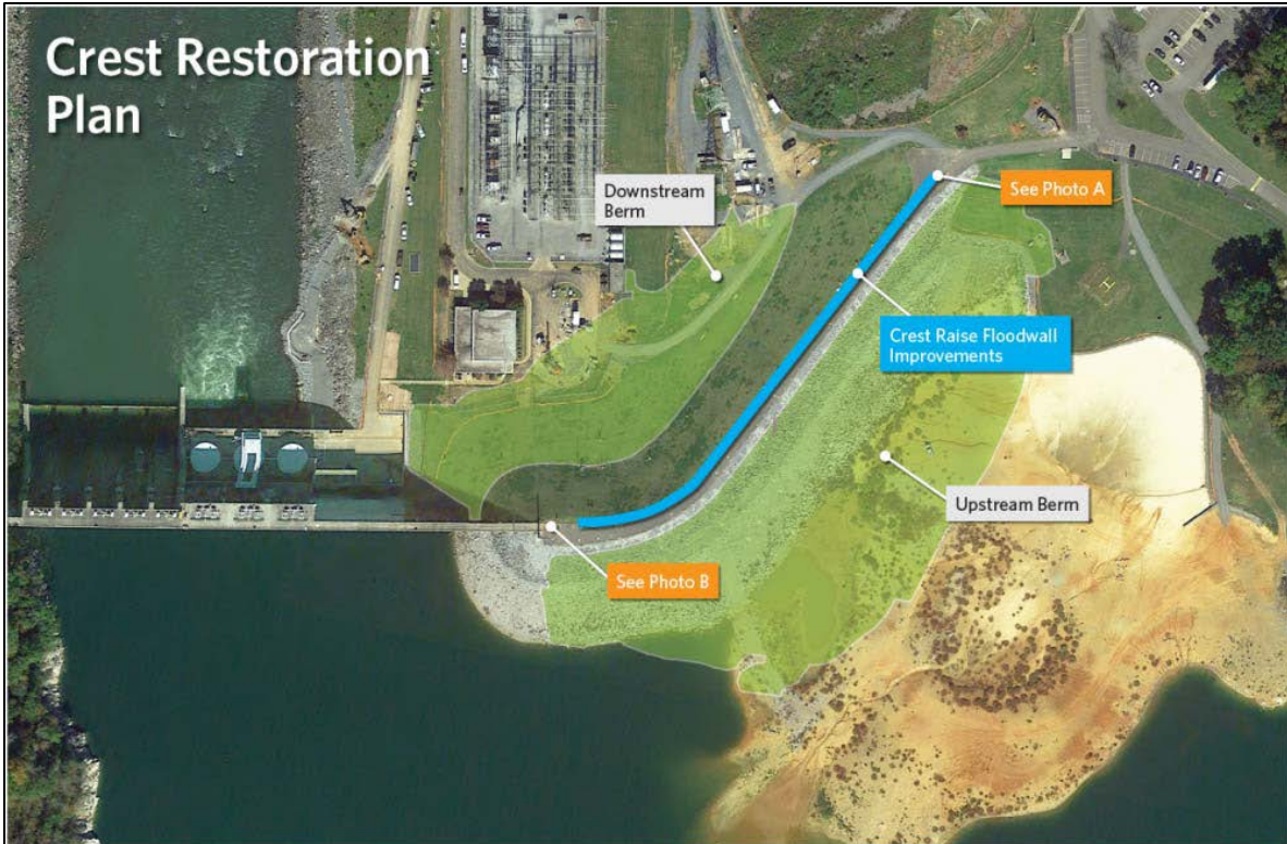
Figure 1. Plan view depicting the location of the proposed floodwall at the crest of the dam.
